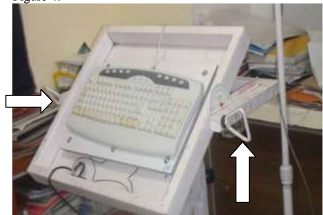
Figure 4: CNC machine panel angle adjustment mechanism
